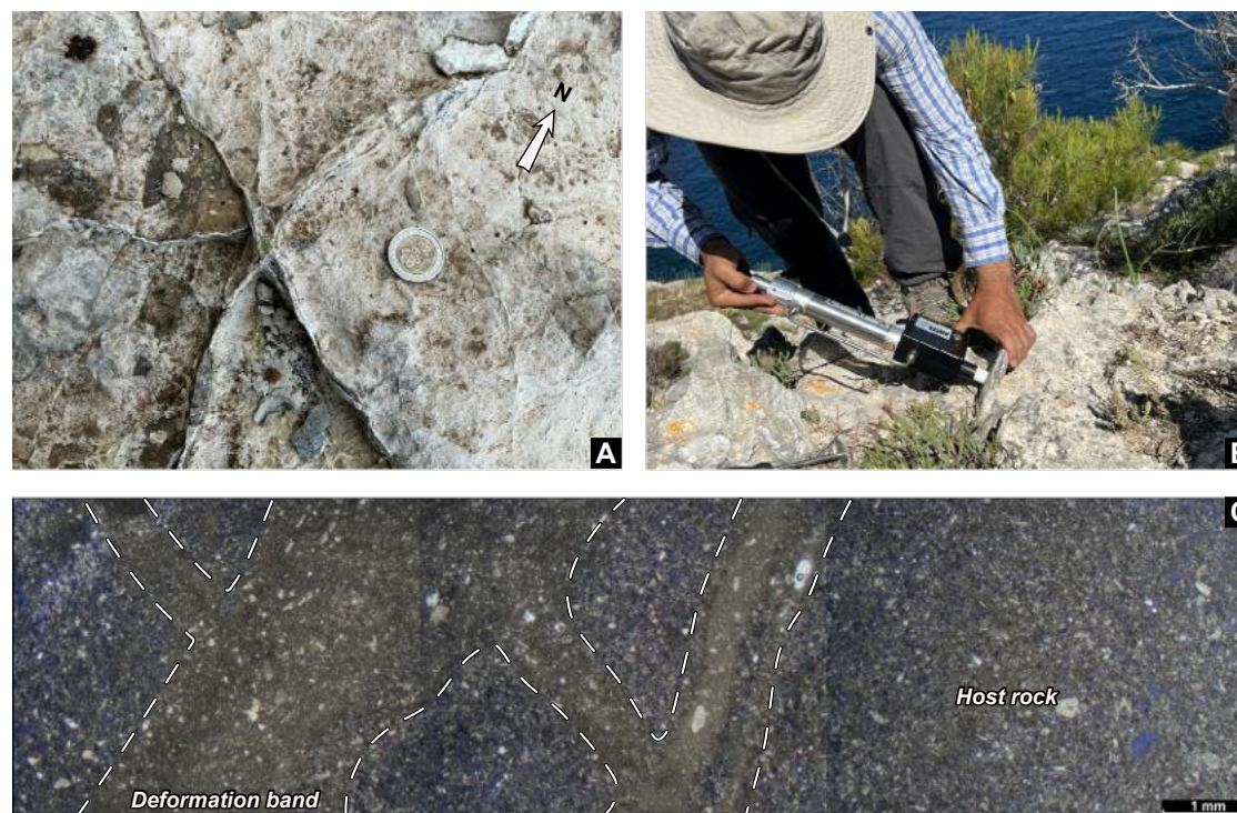
Figure 8. (A) Plan view of the limestones of lithofacies B showing multiple sets of mutually crosscutting deformation bands. (B) In situ measurement of the air permeability along a deformation band. (C) Photomosaic showing microstructural details of deformation bands with cataclastic reduction of particle size and porosity diminishing within the bands compared to the porous host rock.
