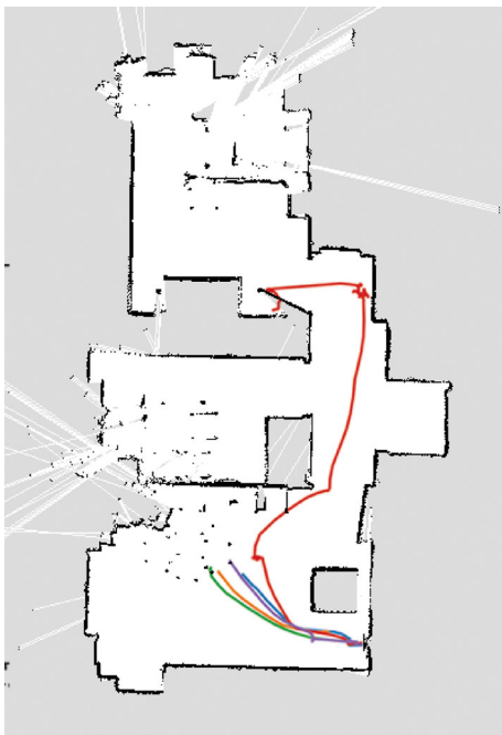
Fig. 7 The trajectories performed by the robot of ITA-2 to perform NPT
