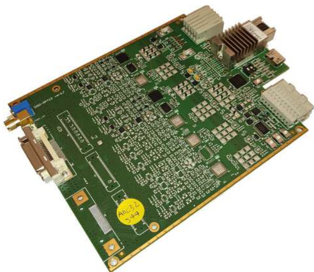
Fig. 2 Photograph of the new Digi-Opt12 v. 3.7 card with two ADC32J44 chips installed
