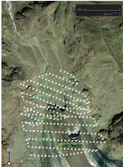
Figure 5. UAV tracks and target distribution - 2020 block.
