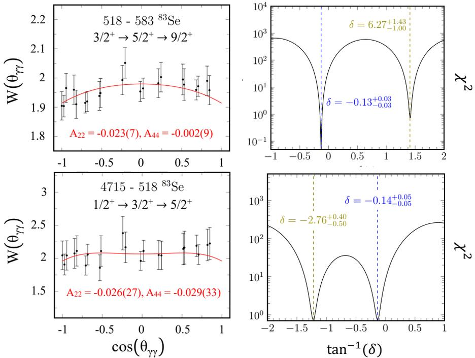
Fig. 3. Left: angular correlation for the 518–583 keV and 4715–518 keV transitions. Right:  $\chi^2$  function for the 518 keV transition mixing ratio evaluation. The  $\delta$  values which minimize the function are reported. The picture is adapted from Ref. [11].
