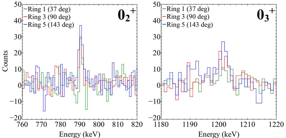
Fig. 1. Portion of the  $\gamma$ -ray energy spectra of  $^{84}\text{Se}$ , as measured by ring 1, 3, and 5 of ROSPHERE, showing the  $0_{2,3}^+ \rightarrow 2_1^+$  transitions of energy 790 (left) and 1200 keV (right), depopulating the  $0^+$  states located at 2244 and 2654 keV, respectively. The spectra are gated on the 1454 keV,  $2_1^+ \rightarrow 0_1^+$  transition.
