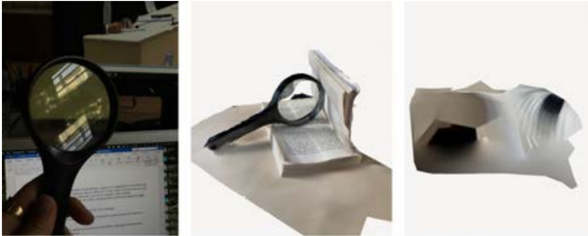
Figure 22 3D scanning tests carried out during the consultation of the documents. From left: photographic image, photogrammetry, Lidar scanner, taken using the Polycam app, and smartphone. Paris, Archives nationales, June 2023. Copyright of the author.
