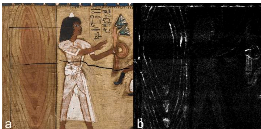
Fig. 7. Casket S. 8213, detail of the son Nekhetef in visible (a) and XRF map of manganese (b).
