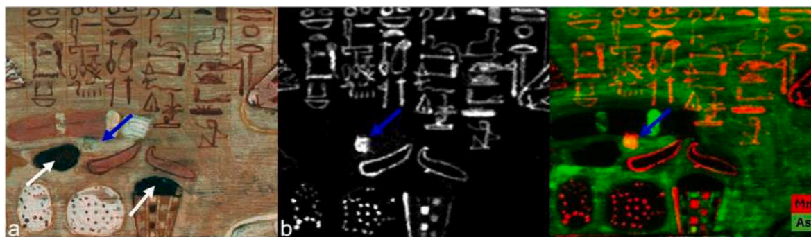
Fig. 10. Casket S.8212; detail of the hieroglyphs in SWIR false color image (a) XRF map of Mn (b) and Mn/As (Red/Green) correlation map highlighting that the black detail, based on manganese black and faintly visible to the naked eye, was covered with an arsenic-based layer of light color in the final step of the realization (blue arrow). White arrows indicate carbon-black areas that remain black in SWIR-FC in contrast to the reddish areas realized with manganese black.
