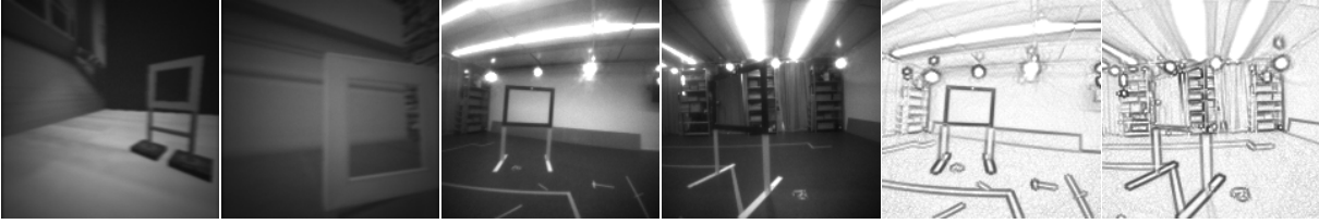
Figure 4.10: Examples of (left) simulated images from \mathcal{S}^{\text{train}} , (middle) real-world robot images in \mathcal{T}^{\text{train}} , and (right) after applying the pencil filter [75].
