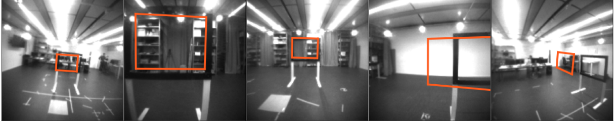
Figure 4.12: Input frames overlaid with gate skeleton (in orange) using the pose predicted by our approach. The model correctly locates the gate (1-3), while failures occur when a large portion of the gate is occluded and for shallow angles (4-5).
