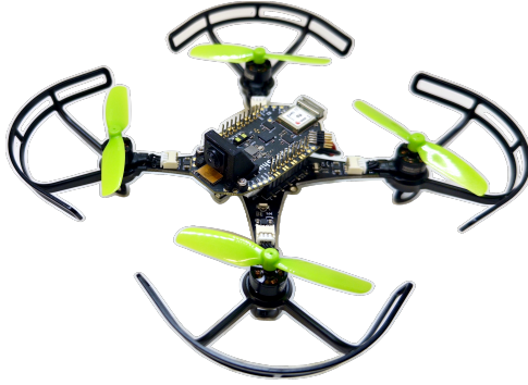
Figure 4.9: The Crazyflie 2.1 Brushless nano–drone used in our experiments.
