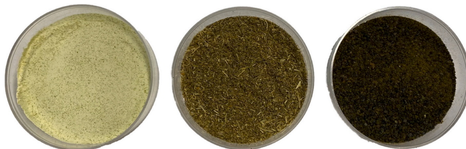
Fig. 3. Images of the commercial flour (left), the dry by-product (centre), and the protein concentrate obtained by the ultrasound-assisted method (right) at the optimized conditions (liquid-solid ratio 20 mL/g, pH 11, amplitude 80 \mu m, time 2 \times 30 min).
