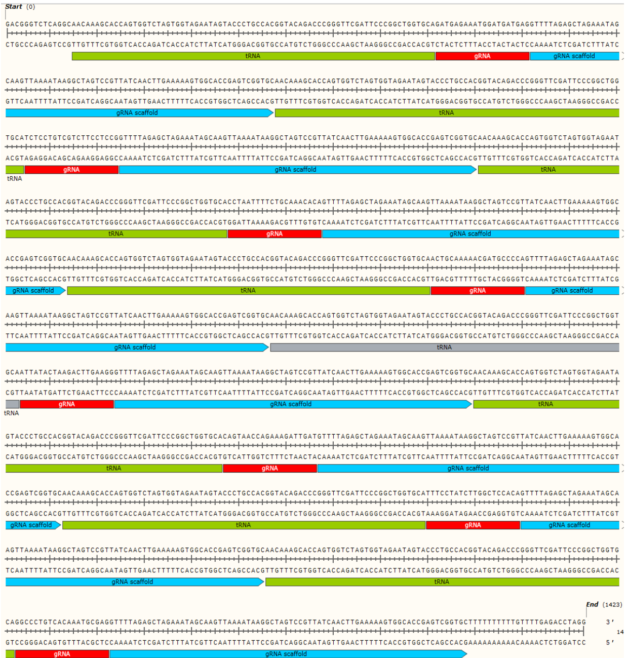
Figure 21. Construct used to generate multiple mutations in PINE1 promoter. The red regions are the actual guideRNA which targets PINE1 promoter, while the blue regions correspond to a scaffold necessary to bind the guide to the Cas9. The blue sequences are tRNA that will be cleaved at both ends.
