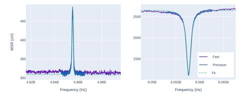
**Figure 3.** Example of two calibration experiments executed using Qibocal on quantum processors. On the left a qubit spectroscopy and on the right a resonator spectroscopy for a qubit hosted at Quantum Reasearch Center (QRC) in Technology Innovation Institute (TII).
