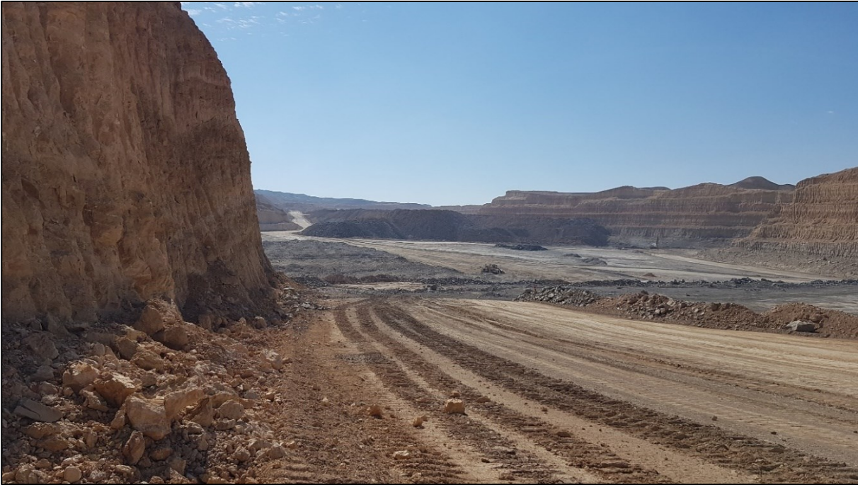
Fig. 5.32 – Overview of Rotem Amfort mining plant highlighting dark-grey outcrops of Ghareb Formation rich in bitumen and the following bitumen-free light-yellow chalky parts.
