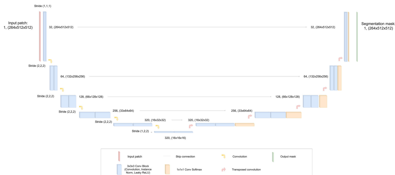
Fig. 6 | A 3D U-Net architecture for airway and lung-lobe segmentation consisting of six encoder stages with feature channels (32, 64, 128, 256, 320, 320) and five decoder stages, all using 3 \times 3 \times 3 3D convolutional kernels. The input shape 264 \times 512 \times 512 reflects the median CT volume size of the preoperative cohort and is
