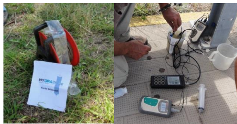
Figure 3.4: a) Hydrasleeve used for water sampling in depth b) Measuring Electric Conductivity, pH, Temperature in situ
