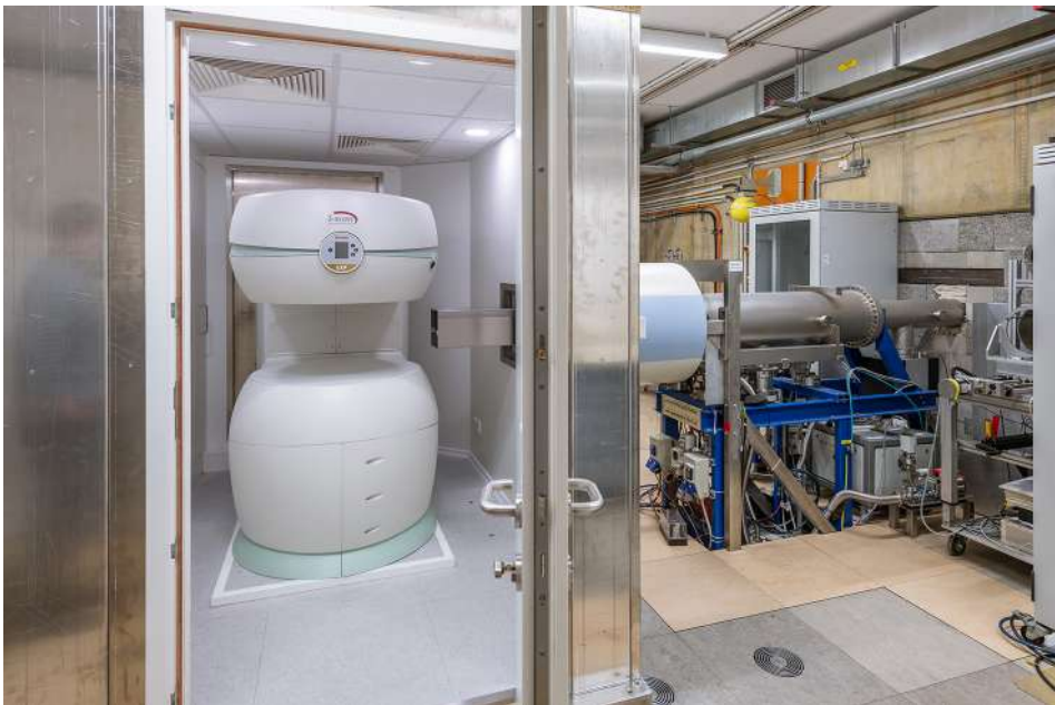
Figure 5.8. Setup of an MRI scanner from Esaote at HIT's experimental place.
