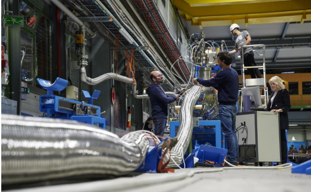
Figure 3. Short prototype of the High Luminosity LHC Superconducting Link system during first operation at CERN. Courtesy Amalia Ballarino (CERN).
