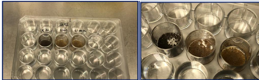
Figure S1. Virucidal assay performed in a 24-well plate. Different resins were dispensed into individual wells and exposed to virus suspensions for the selected contact time at room temperature. Each well contained 100 mg of resin and 500 \mu L of viral suspension.
