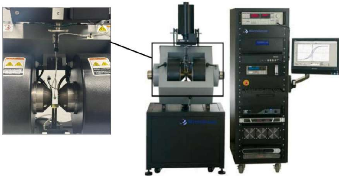
Figure 3.12: Vibrating sample magnetometer (VSM) MicroSense EZ7. Top left: sample mounted on the quartz rod and positioned between the instrument dipoles (image by Ottavia Gigliotti).
