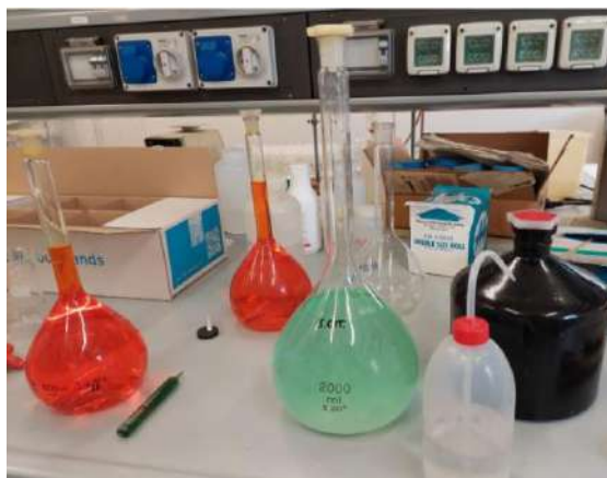
Figure 3.5: Reagents used for the analyses. On the left potassium dichromate (orange); on the right ammonium iron(II) sulfate solution (green).
