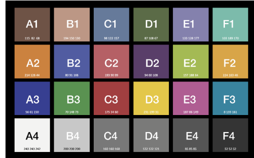
Fig 1. The target Calibrite ColorChecker Classic.
