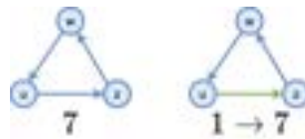
Fig. 4.3: On the left, a static close directed triad among the vertices u, w and z . Number 7 corresponds to the ID assigned to each kind of triad. On the right, is the corresponding closing temporal triad. From the open triad (blue link) by the insertion of the green link (u, z) we move to the close triad 7. 1 \rightarrow 7 indicates that we move from the open triad with ID 1 to the closed triad with ID 7
