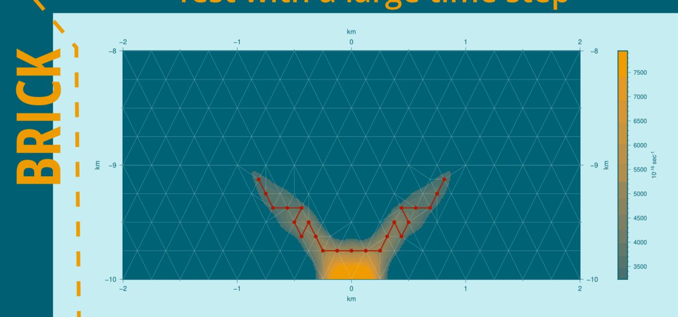
We place a **brick** with different viscosity at the bottom of a viscoplastic system and push the sides. The system immediatley breaks generating two **shear bands**. The algorithm generates a linear fault that approximates the geometry of the shear bands and refines the grid.
