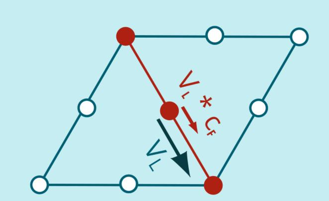
Coupling factor applied to compute velocities on one side having velocities on the other side
