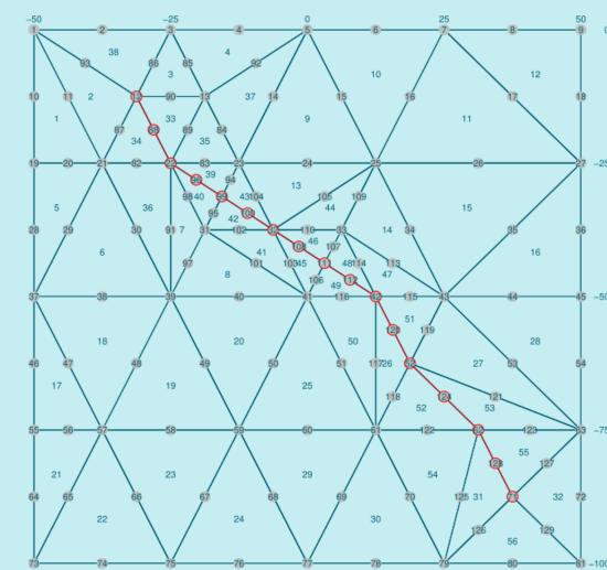
When the fault cuts the grid, a mesh refinement is necessary.
