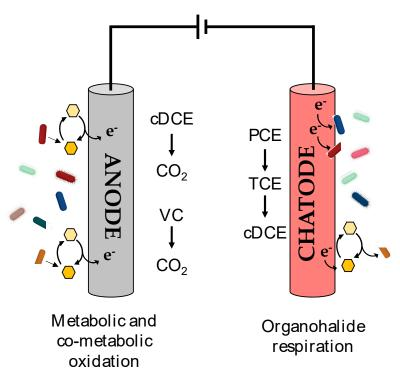
**Figure 6.** Illustration of a bioelectrochemical cell with aerobic and anaerobic biotransformation of chloroethene mechanisms.
