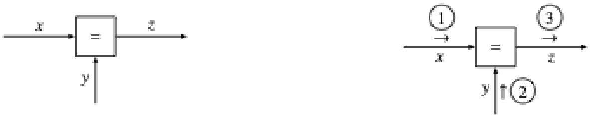
Figure A.3: FFG representation (left) and message passing schedule (right) for an equality constraint node.
