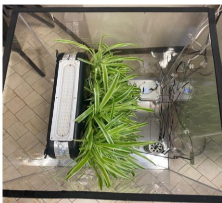
Figure 1: Top view of the chamber with the biofilter module, the heater and the NETPID sensor.
