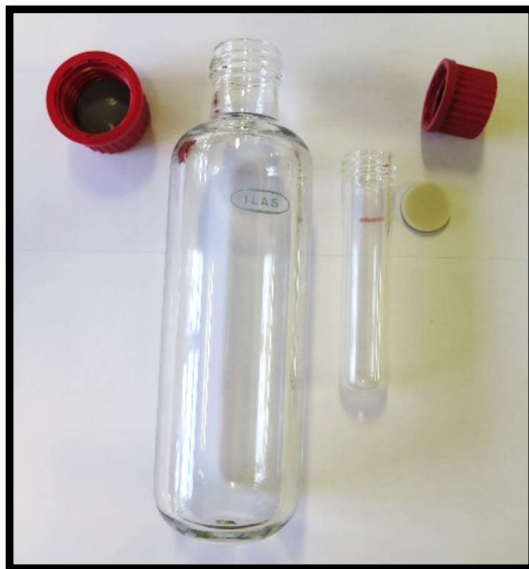
Fig.4. Left : Pressure bottle used in the large-scale reaction under conditions B. Right : Pressure tube used during our study.
