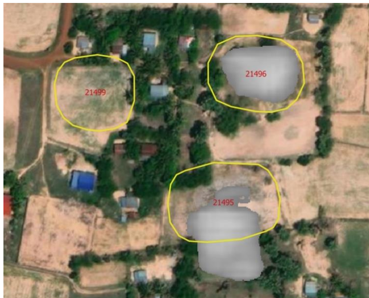
Figure 19. Actual (yellow) and predicted (grey) reservoir shapes in a test region near Angkor Wat.
