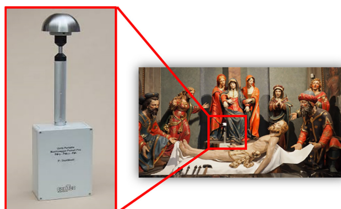
Figure 11. P-Dust Monit positioned in one of the main chapels close to the sculptural group of the Deposition .
