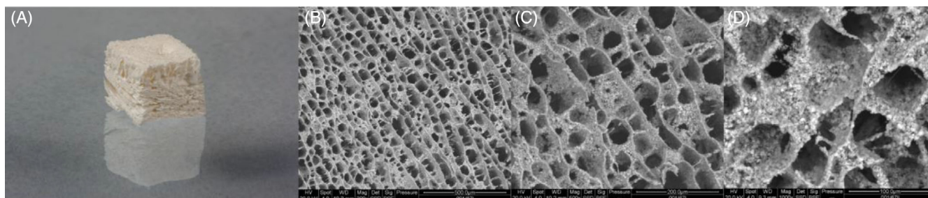
FIGURE 1 (A) OSSIX™ Bone Sponge-like, porous, space-maintaining block. OSSIX™ Bone appears in the SEM images as an organized honeycomb-like spongy structure where small hydroxyapatite particles are randomly dispersed within and on the solid collagen wall structure of the product. (B) \times 200 ; (C) \times 500 ; (D) \times 1000 .
