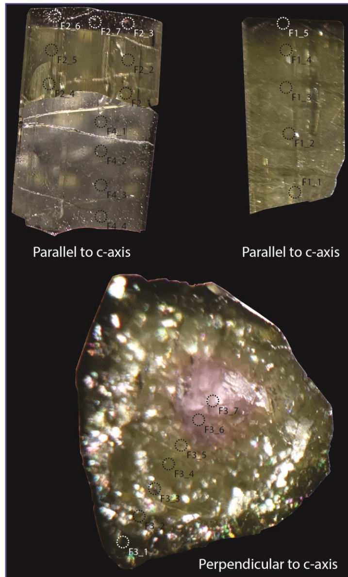
Figure 7-7 Traverses on tourmaline crystals from the LCT pegmatites miarolitic cavities. At the top, black-capped tourmalines analyzed along the C-axis, at the bottom a watermelon tourmaline analyzed perpendicular to the C-axis.
