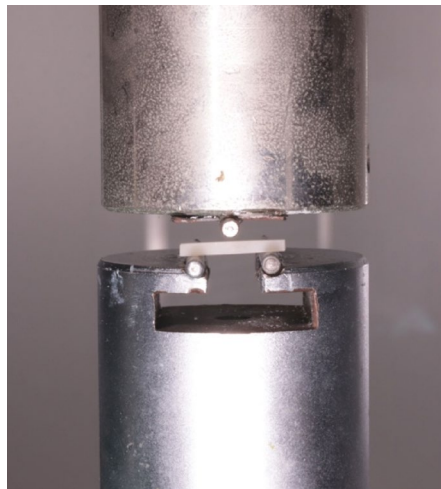
Fig. 6. Universal mechanical testing machine including the setup for the 3-point bend test and a bar specimen positioned in the center of the testing area.
