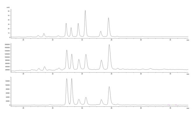
**Figure 2.** Chromatographic profiles at 350 nm of the SFE1 sample with the corresponding total ion current in the negative ionization mode and the EI at 315 m/z corresponding to the aglycone for the isorhamnetin derivatives; (1,2) quercetin 3-O glucosides; (3,4) isorhamnetin 3-O glucorhamnosides; (5,6) isorhamnetin 3-O glucosides; (7,8) isorhamnetin acetyl hexosides.
