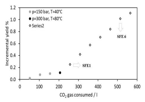
**Figure 1.** Supercritical CO<sub>2</sub> extraction kinetics: each point represents the incremental yield (% mass extract/mass biomass) detected over the time and, hence, over CO<sub>2</sub> consumption.
