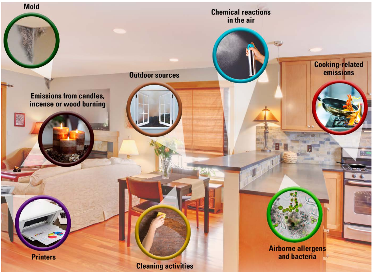
Figure 3. Summarizes all the main sources of indoor particulate matter (PM): cooking, cleaning, combustion, biological contaminants (i.e., mold and bacteria), printers, chemical reactions, and outdoor infiltrations. The image can be found at www.epa.gov/iaq .
