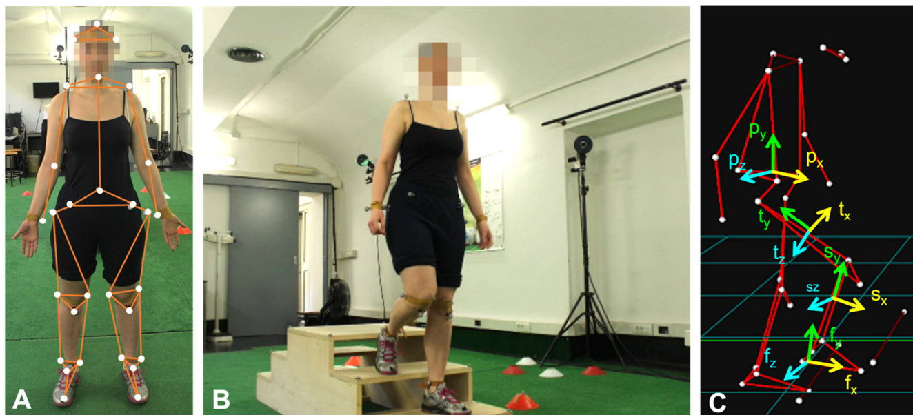
Figure 1. Experimental setup. (A) Reflective markers placement; (B) wooden stairs and participant performing the task; (C) pelvis and lower limbs reference frames (superscript legend as follows: p, pelvis; t, thigh; s, shank; f, foot).
