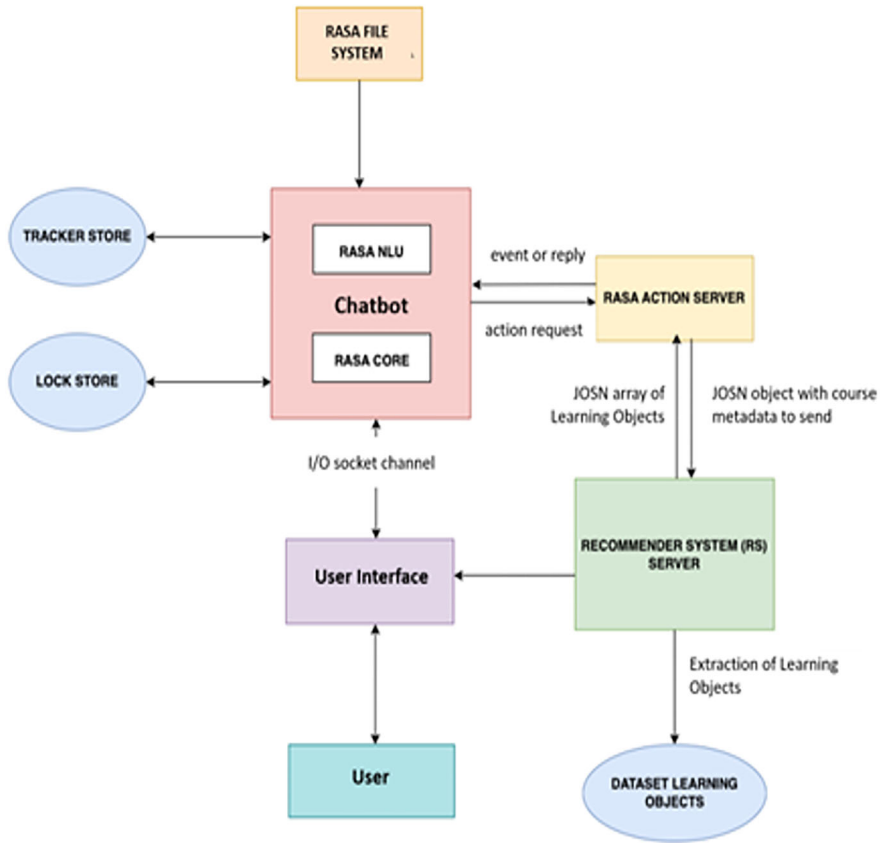
Fig. 1 General architecture of the e-learning platform
