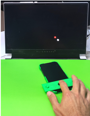
Figure 1: The experimental setup, as used in object following. The user controls the gray nail-like object with the goal of staying as close as possible to the red dot. The iPhone simulates the button using its Taptic Engine, delivering vibrotactile pulses.
