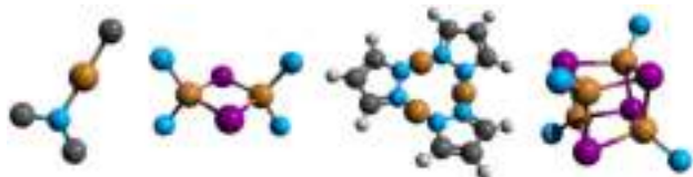
Fig. 2 Schematic structures of the most representative monomers (labelled either 1.x y , with x being the NHC and y the amide ligands, or 1.n ), dimers (labelled 2.n ), trimers (labelled 3.n ) and tetramers (labelled 4.n ), where n is the compound number within a given category reported in the review. Colour code: brown = Cu; purple = halogen; light blue = nitrogen.
