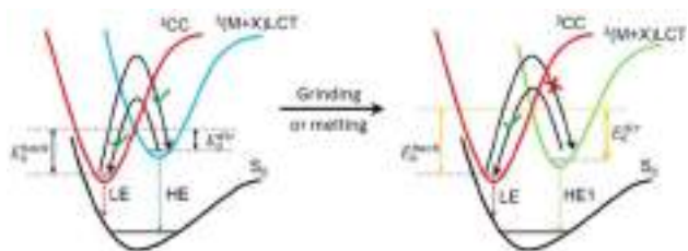
Fig. 23 Simplified diagrams explaining the thermo- and mechano-chromic luminescence of pristine (left) and fully amorphized (right) 3.30 . E_a^{\text{dir}} and E_a^{\text{back}} represent the energy barriers for the direct and reverse population, respectively, from the ^3(\text{M} + \text{X})\text{LCT} to the ^3\text{CC} states. Reproduced with permission from ref. 138. Copyright 2021, John Wiley and Sons.
