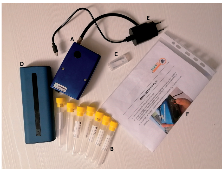
Figure 4. Air quality monitoring participation kit including BC sampler (A), filter storage tubes (B), replacement filters (C), external battery (D), battery charger (E), and the information sheet (F).
