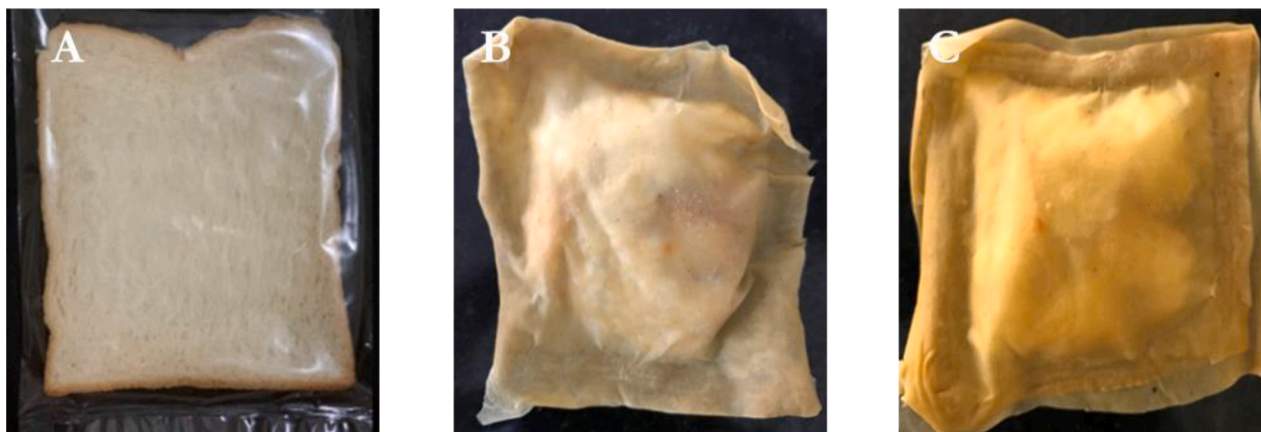
Fig. 1. A) Bread sample packed in PE films, B) Bread sample packed in BPT film, C) Bread sample packed in Bioactive BPT film.
