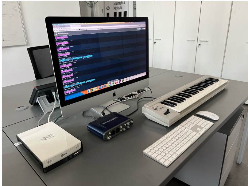
Figure 8: Testing the Web MIDI Monitor with a physical MIDI setup.
