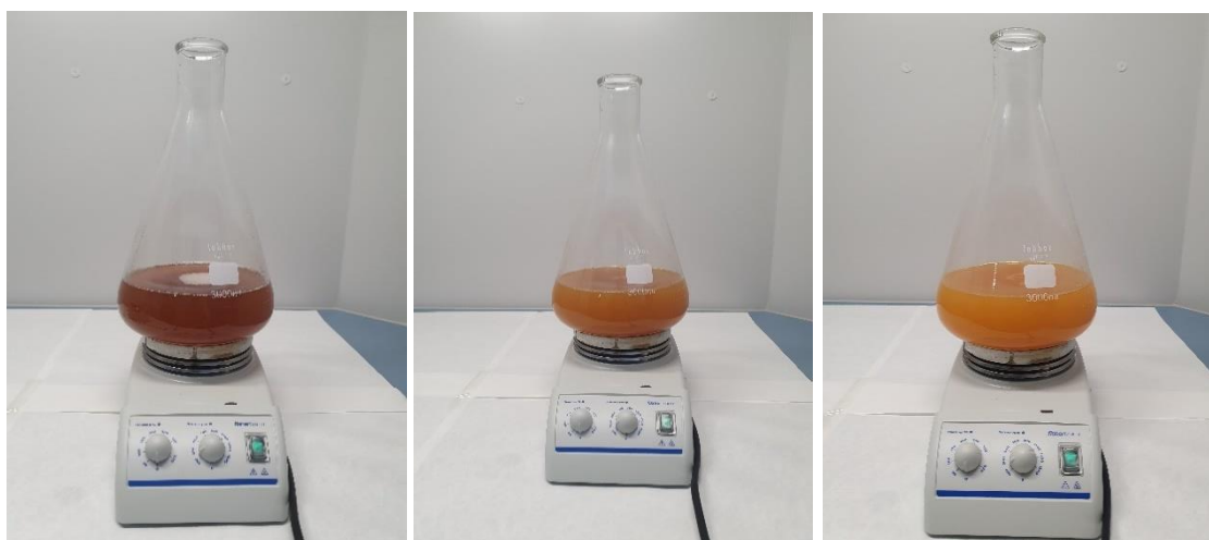
Figure 2.9. Formation of the corresponding hydroxides and oxides of nanometric size during time.
