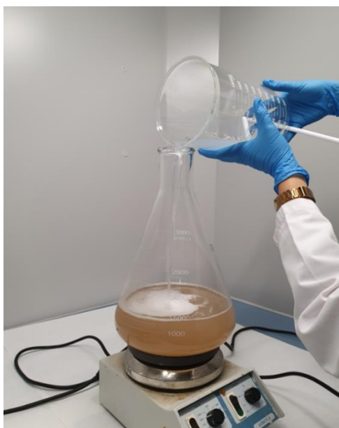
Figure 2.8. Addition of the solution containing the base to the microemulsion containing the precursors.
