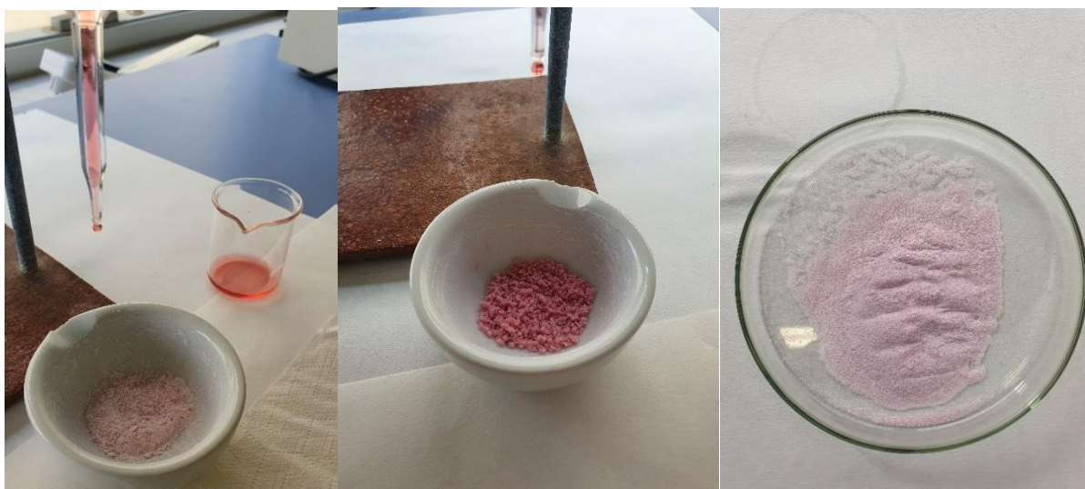
Figure 2.3. Experimental setup for the incipient wetness preparation method and resulting aspect of the cobalt precursor powder after pouring the whole solution.
