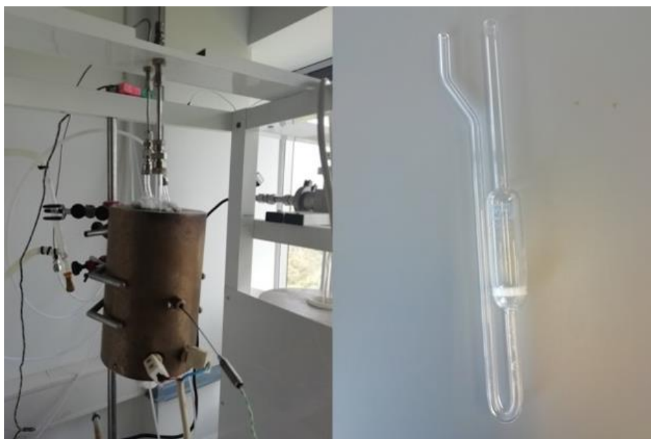
Figure 2.12. Preparation system for the reduction of the mixed oxides.
