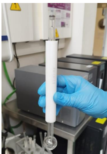
Figure 2.13. BET reactor wrapped in a heating coat and containing the sample.
