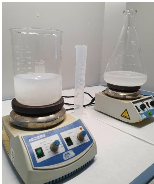
Figure 2.7. The two separates inverse microemulsions containing the precursors and the base, respectively.
