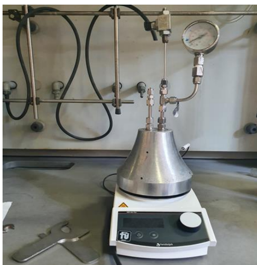
Figure 2.16. The autoclave used for the reactions, inserted in the heating bell with a thermocouple on the rear side, placed on the heating plate.
