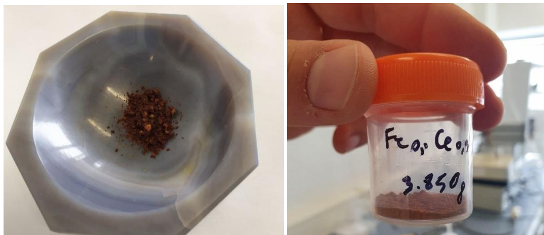
Figure 2.11. Dried orange slime after the oven treatment (110°C), crushed into a fine powder.
