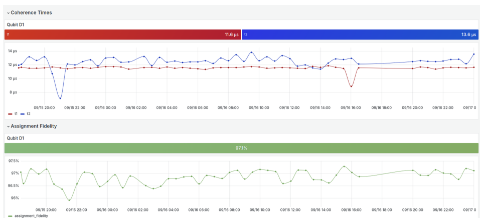
Figure B.4.: Monitoring of coherence times and readout fidelity using Qibocal.
