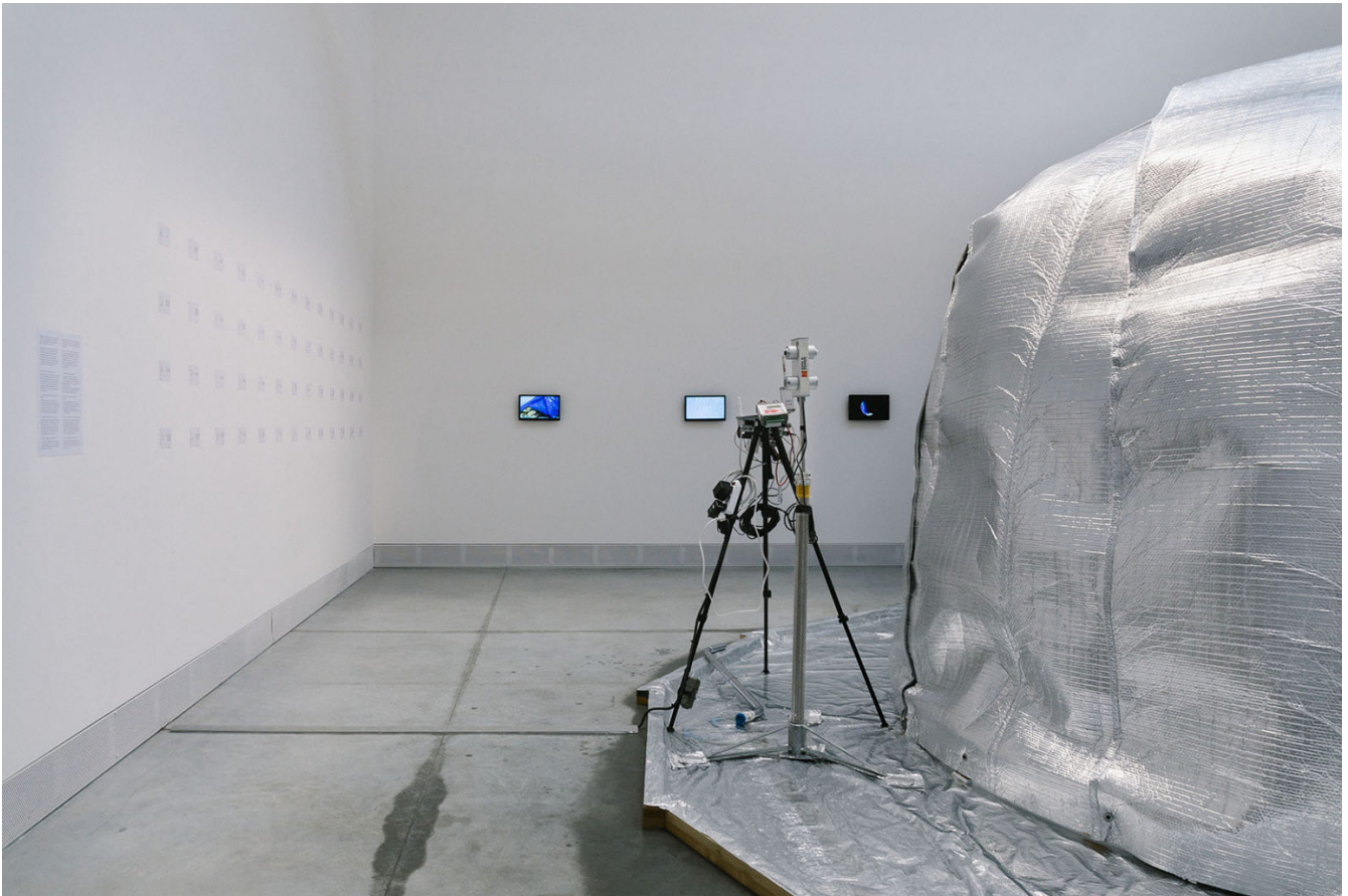
Figure 2 - The automatic weather station ( AWS_{Biennale} ) installed near the "Melting Landscape" work.
