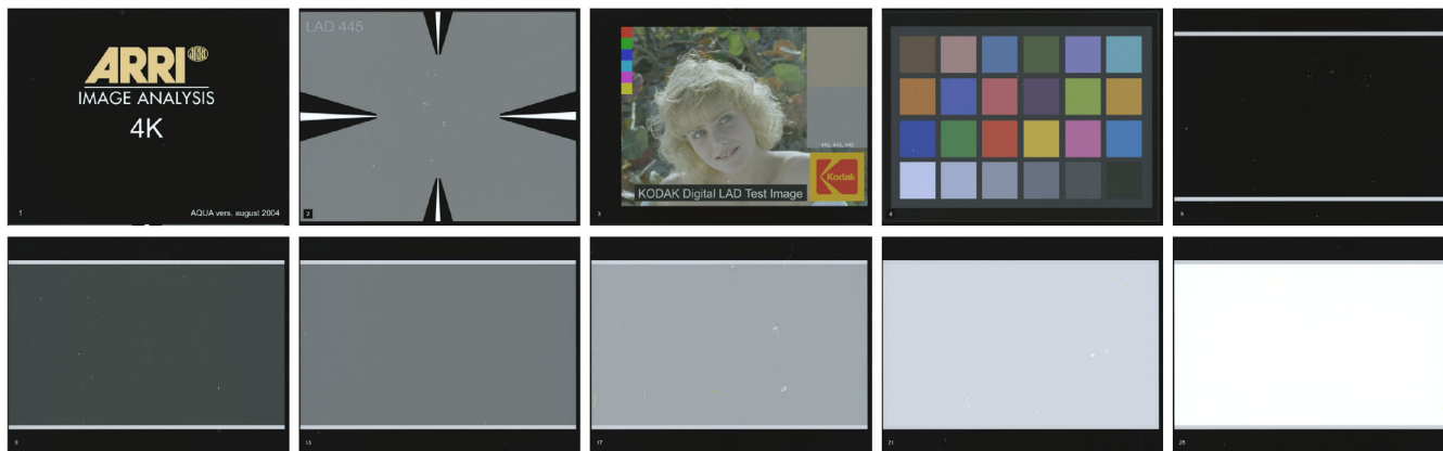
FIGURE 5 Representative frames of the ARRI AQUA test leader. The reported frames are Frame 1, 2, 3, 4, 5, 9, 13, 17, 21, and 25 digitized using scanner 1.
