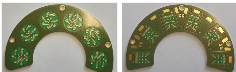
Figure 2.25: Photograph of the flange with the rigid PCBs required to interface the electrical feed-through connectors with the block-FETs, which host the input transistor of the charge-sensitive preamplifier and the feedback network.
