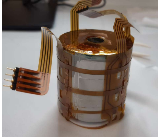
Figure 2.20: Flexible PCB connecting the electrodes of the detector. Each arm of the PCB lies on the doped surface and is held in place by three long polyimide strips wrapped around the detector itself.
