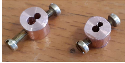
Figure 2.16: Photograph of the copper clamp used for the high-voltage connection.
