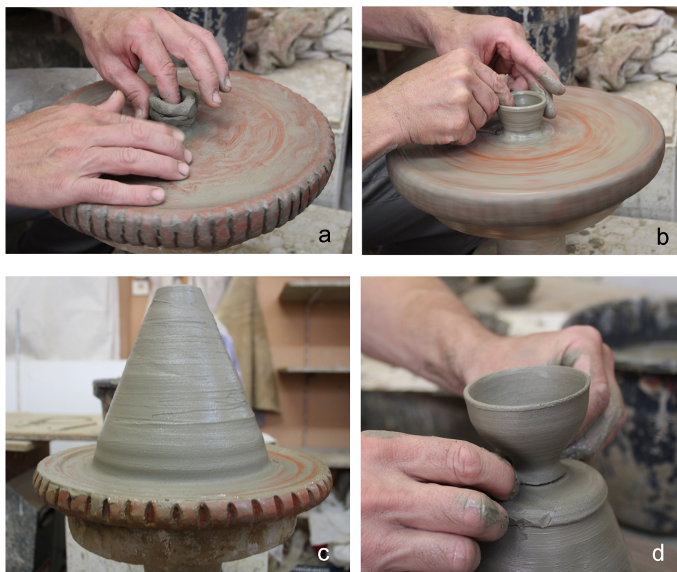
Figure 2. The two ceramic forming techniques used for the experimental work: wheel-coiling (a,b) and throwing off-the-hump (c,d).
