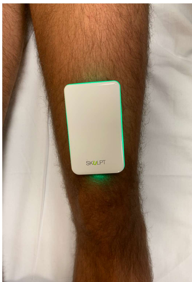
Figure 2. Skulpt Chisel™. This figure shows how to correctly place the Skulpt EIM device on the anterior aspect of the distal third of the thigh.
