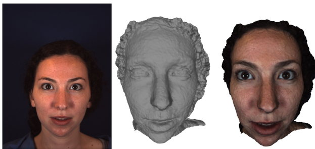
Figure 4: An example of a BP4D+ record. From left to right, a frame’s 2D RGB texture, plain mesh and RGB mesh.
