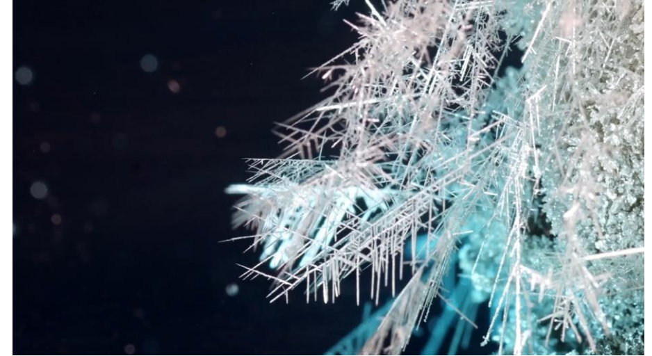
The growth of silver crystals on the surface of copper from a solution of silver nitrate. Bilovitskiy CC BY-SA 4.0 Deed
