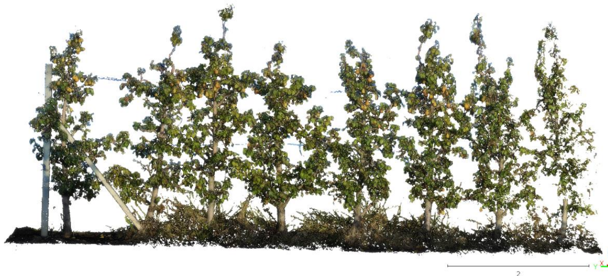
Figure 2. Point cloud created with digital terrestrial photogrammetry with about 82 million points.
