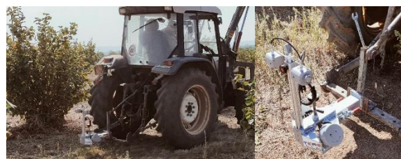
Figure 1. MECS-VINE multi-sensor mounted behind the tractor prospecting the hazelnut grove
