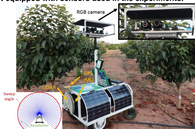
Figure 1. Scouting robot equipped with sensors used in the experiments.
