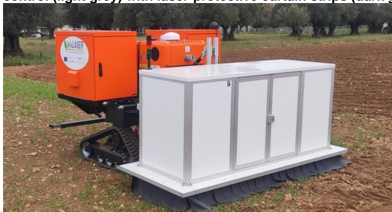
Figure 1. Autonomous mobile robot platform with adapted laser-irradiation unit for laser-based weed control (light grey) with laser-protective curtain strips (dark grey) attached to the lower edge [3].
