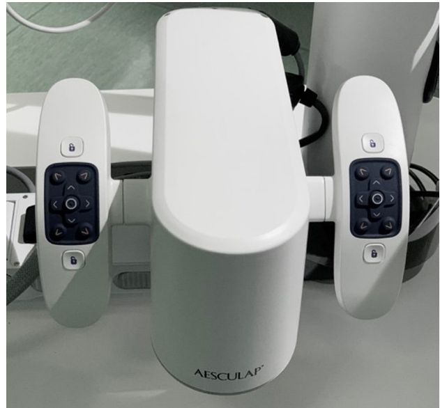
Fig. 2 Two different control areas are located on the right and the left side. The surgeon can choose the position of the commands in the 2 areas in order to move the robotic arm, to select the light intensity and to check the focus. Moreover, it is possible to take pictures and videos and save the position of the arm in the space
